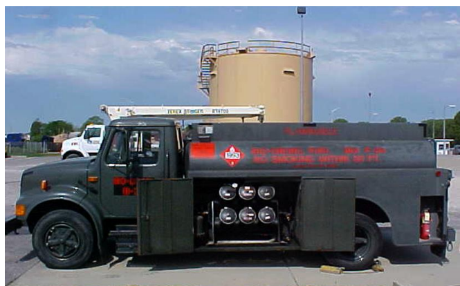
U.S Air Force installed Model 6175 (78 gpm max.)
