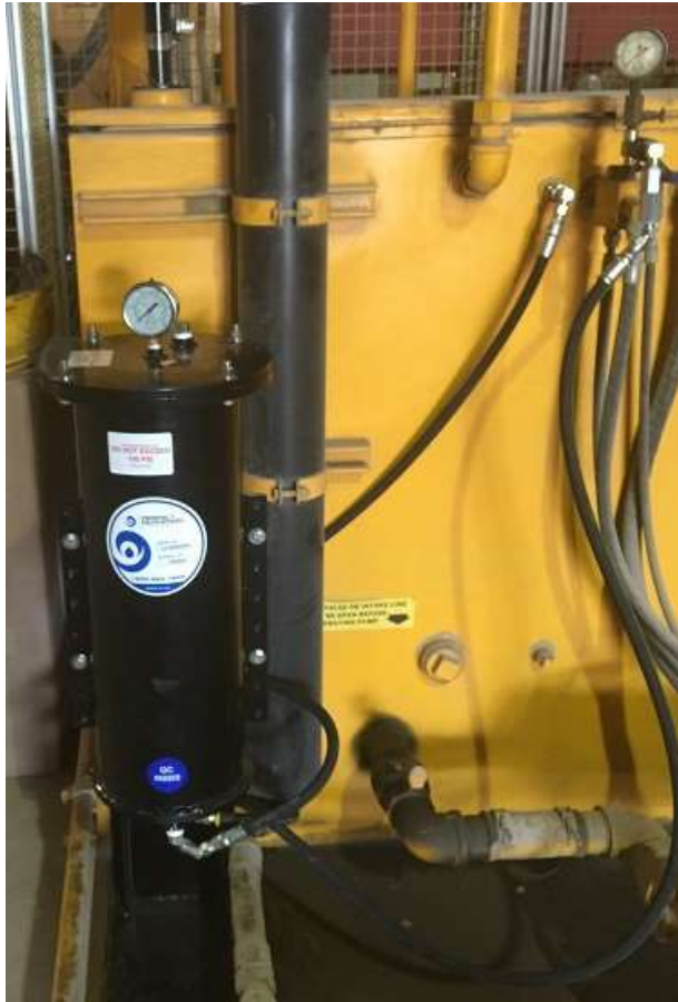
Model U-1000H-PRV with floor stand. The system keeps the hydraulic fluid ultra clean and water free. This customer has not changed hydraulic fluid in over five years and has not had any failures or downtime related to dirty fluid.
