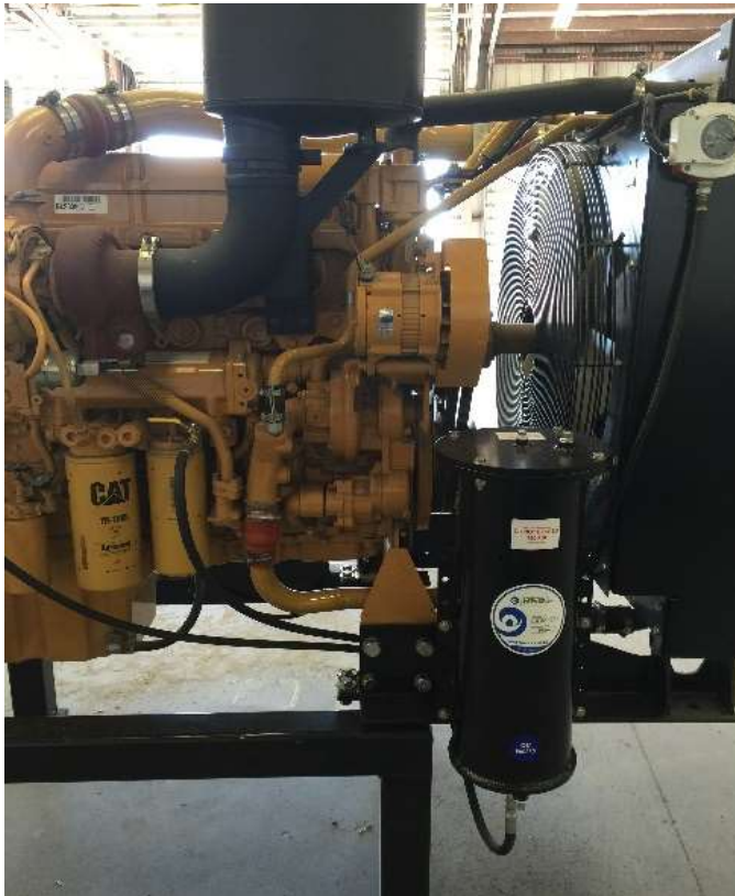
Model U-1000L installed on a CAT engine. The customer was changing engine oil every 250 hours and with the added high quality filtration they are changing oil every 1,000 hours. Oil analysis determined the new service interval
